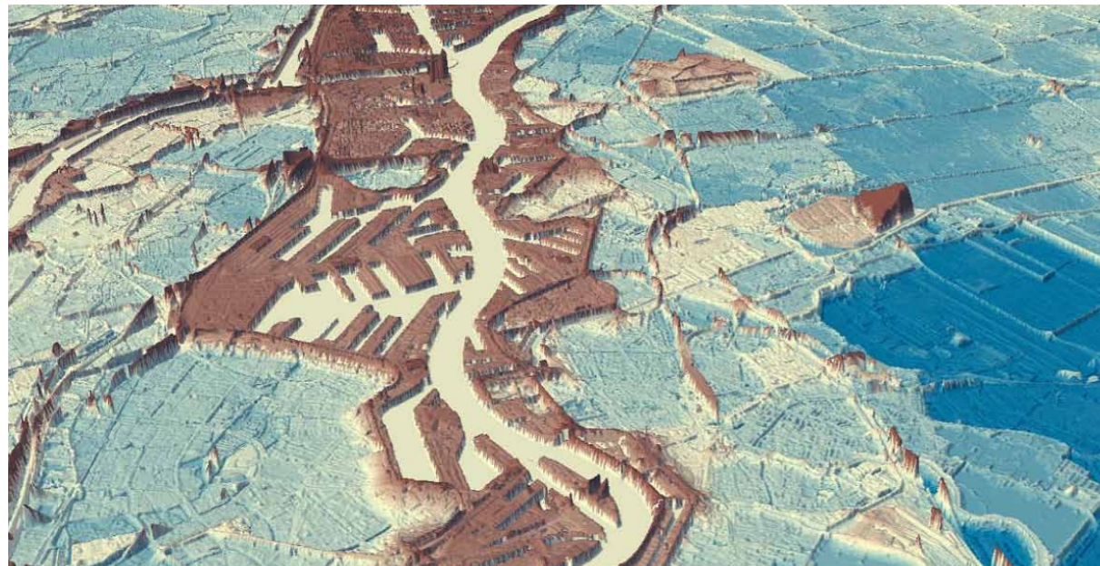
3D model representing the height of land in Rotterdam. The inner-dike area is lower than the river. (source: I. Bobbink, TU Delft)
