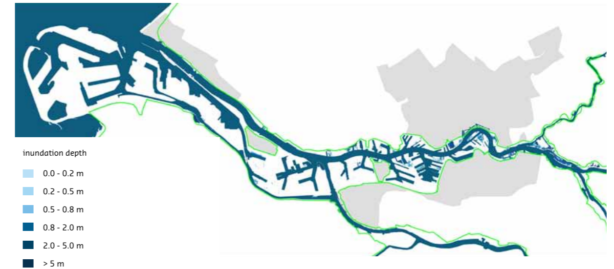
Map 1: Outer-dike flooding in Rotterdam in 2015 (source: Deltares) with a frequency of 1 x 1,000 years
