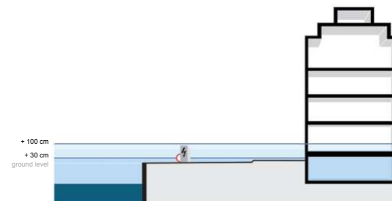
The historic outer-dike areas are the most vulnerable to damage by flooding
