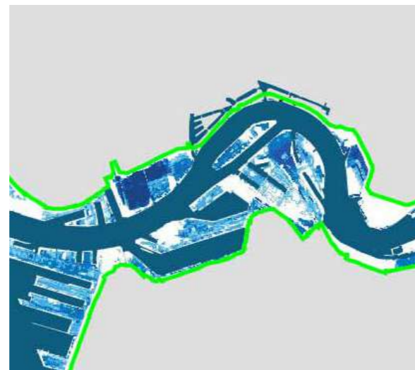
Zoom: Rotterdam centre, flooding in 2100 (W+ climate scenario with a frequency of 1 x 1,000 years)
